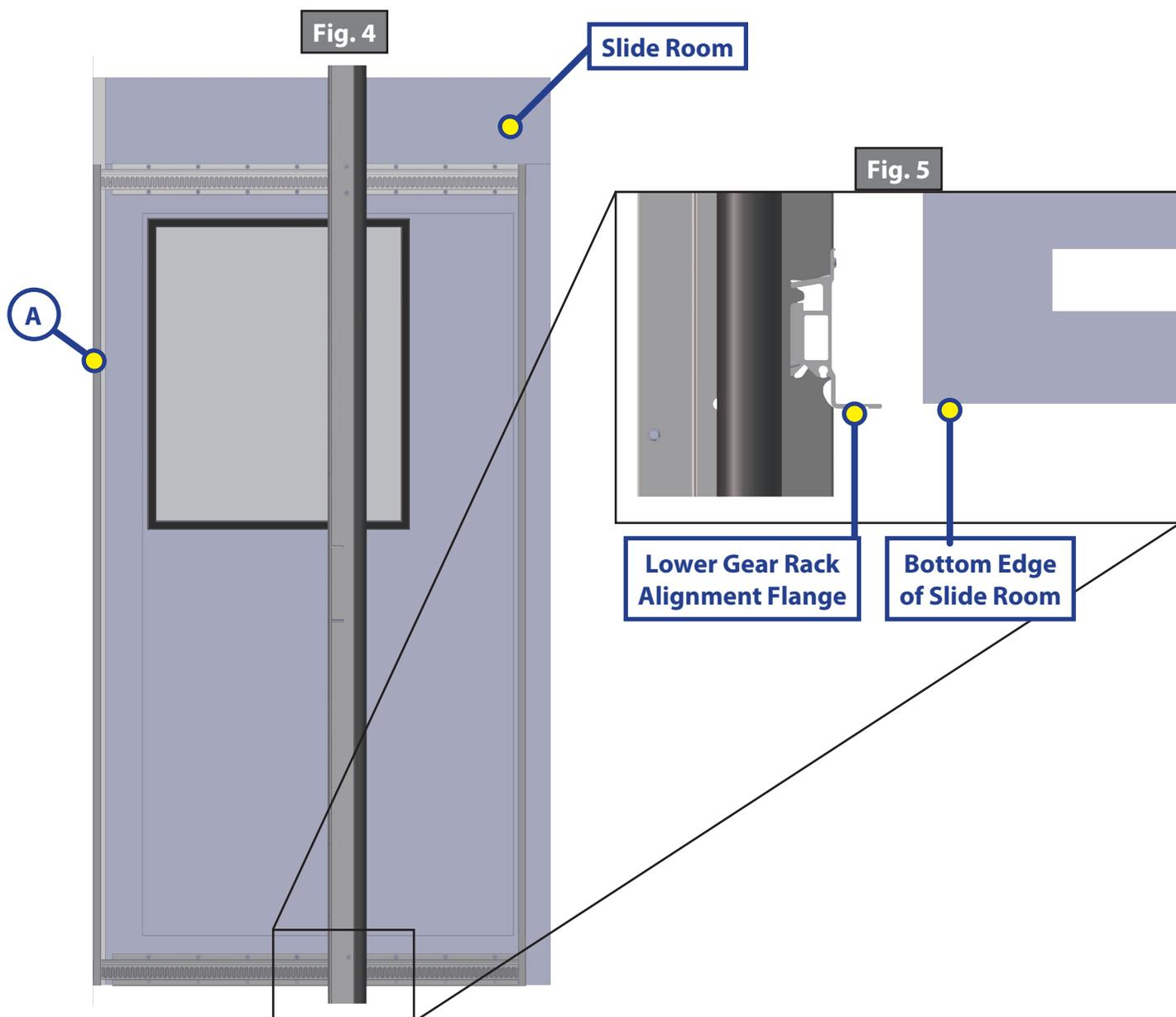
20. Push the bottom gear rack tight against the bottom of the slide room and put a screw into each end of the gear rack.
