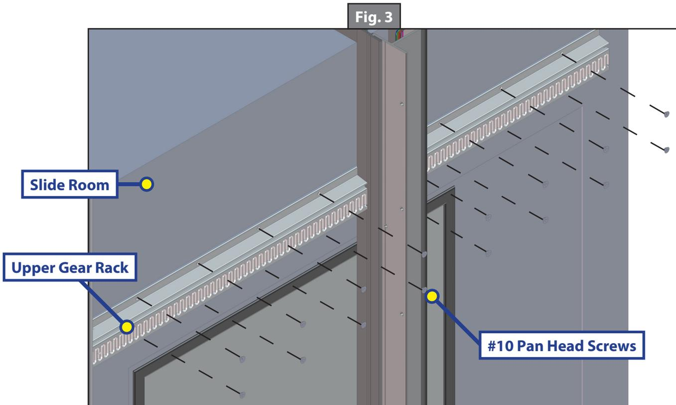
11. You may need to pry the gear racks away from the sides of the slide room with a flathead screwdriver or putty knife. Do this carefully so you don't damage the finish on the side of the slide room.
